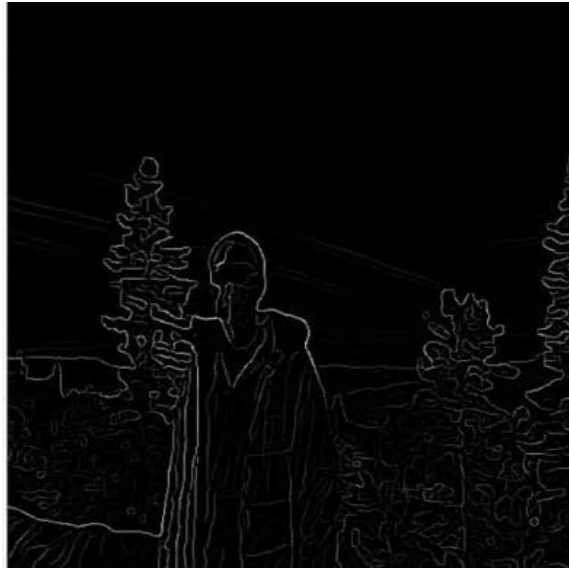
Figure 3.4: output image produced by canny edge detection
