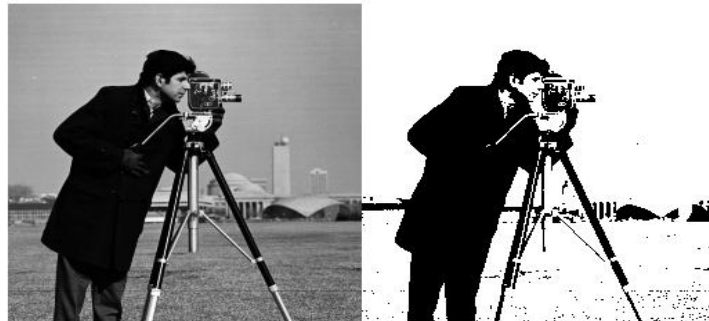
Figure.4.1: Binarization of a gray-scaled image using thresholding method
